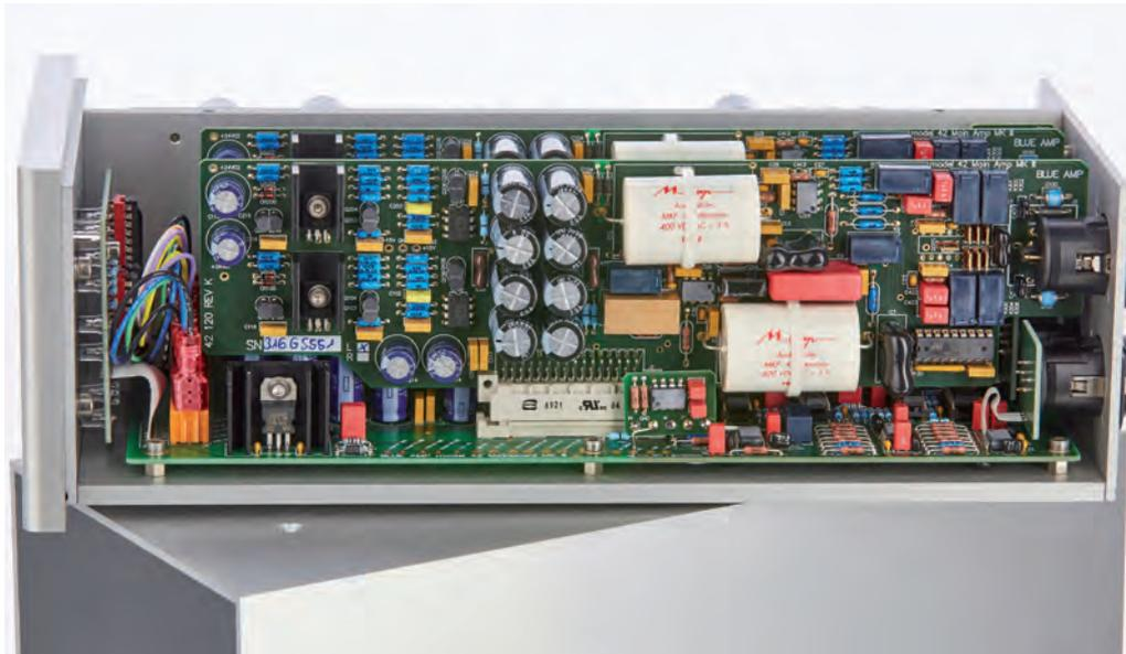
The signal processing circuit board – here to be seen the one of the left channel - is equipped with components of highest quality from i.e. Vishay and Mundorf
