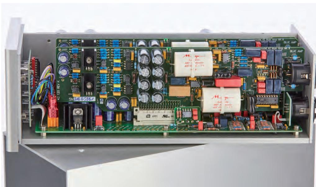
The signal processing circuit board – here to be seen the one of the left channel - is equipped with components of highest quality from i.e. Vishay and Mundorf
