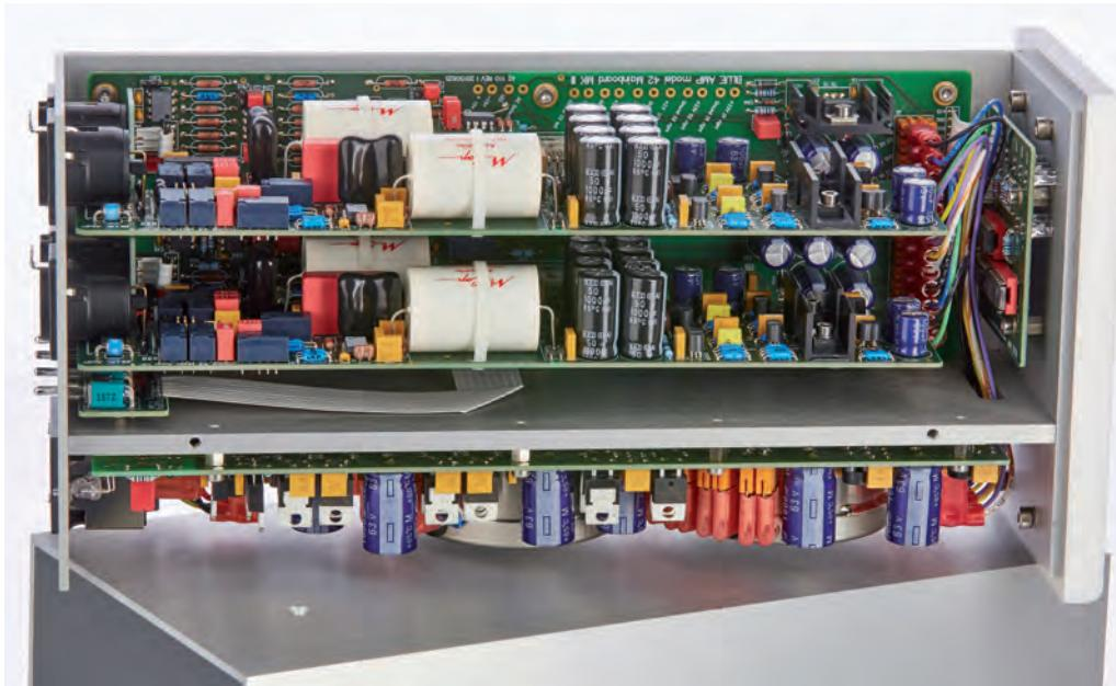
*The power supply circuit board is separated by a thick aluminum plate from the two boards for signal processing and those carrying the controller section*
