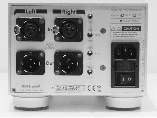
Rolf Becker's opinion, the design of his phono amps makes a shielding of the input cable obsolete, so that their length may even extend up to several meters, thus making a ground socket dispensable. Oh, and yes, the mains phase is also displayed. The change towards a higher quality and therefore much more expensive power cord, the Model 42 MK III acknowledges sonically in a positive way.
